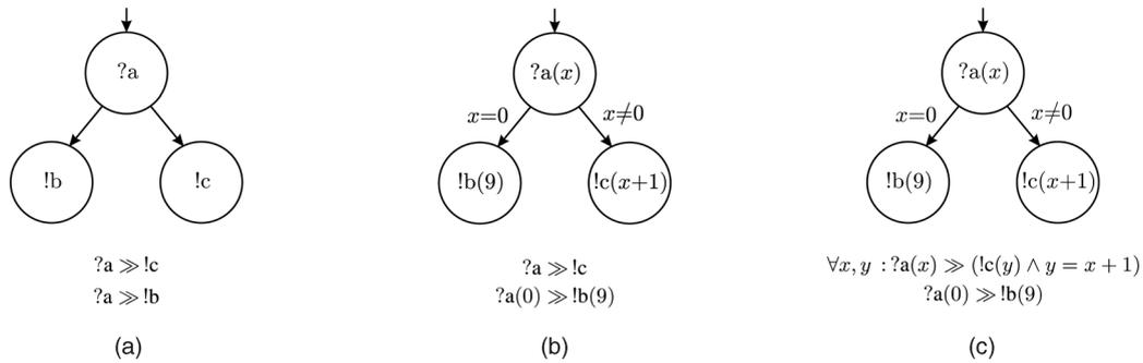
Fig. 1. Workflow modeling with various degrees of data-awareness. (a) Propositional workflow, propositional properties, (b) data-aware workflow, propositional properties, and (c) data-aware workflow, data-aware properties.
