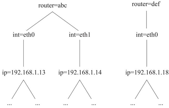
**Figure 4. An excerpt from a configuration of a VPN**
